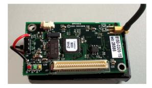
Atmel ATMEGA128L Program Flash Memory Measurement (Serial) Flash **Configuration EEPROM** Serial Communications Analog to Digital Converter 10 bit ADC
