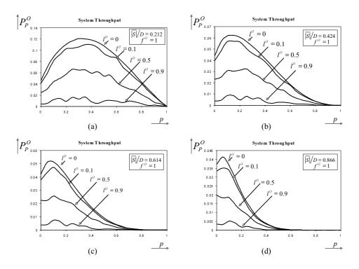
Fig. 10. System throughput (P) simulation results as a function of p for different values of  $l^O$  under no topology control (traditional omni-directional antennas).
