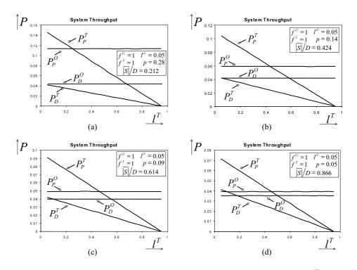
Fig. 13. System throughput (P) simulation results as a function of  $l^T$  for both policies with or without topology control.
