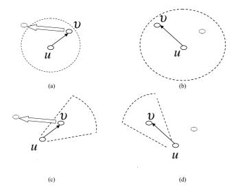
Fig. 7. Node v is moving (white arrow) under topology control. Adaptation of the transmission power, (a) and (b), takes place or adaptation of the transmission angle, (c) and (d). Transmission  $u \to v$  (black arrow) continues and it is not terminated.
