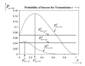
Fig. 4. Probability of success for transmission  $u \to v$  in one frame  $(P_{u\to v})$  as a function of p.
