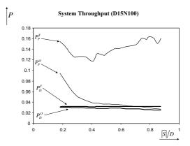
Fig. 11. Maximum system throughput (P) simulation results for both policies, for different values of the topology density  $\overline{|S|}/D$ , when traditional omni-directional and smart antennas are used (nodes are not moving).
