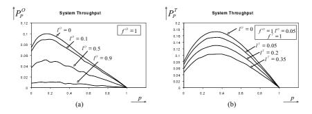
Fig. 8. System throughput under the Probabilistic Policy for the network depicted in Figure 3 (a) under no topology control and (b) under topology control.
