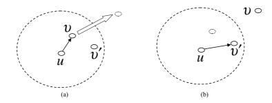
Fig. 6. Node v is moving (white arrow) under no topology control (omni-directional antenna). Transmission  $u \to v$  (black arrow) is terminated and, after a certain number of frames, transmission  $u \to v'$  is started.
