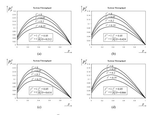
Fig. 12. System throughput  $(P_P^T)$  simulation results as a function of p for different values of  $l^T$  under topology control (smart antennas).
