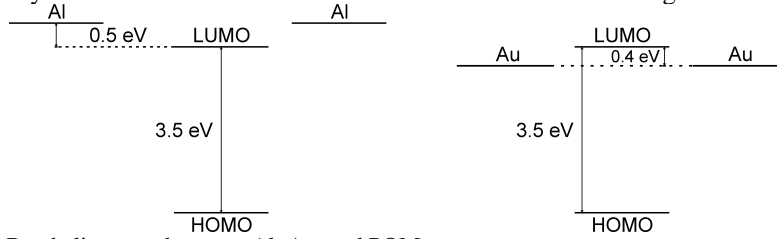
Fig. 3. Band alignment between Al, Au, and POM.
