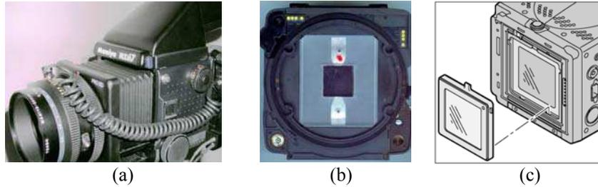
**Figure 7.** (a) medium format camera Mamiya RZ67 Pro IID, accepting either film or a digital back. (b) film holder with MLA attached (c) digital back Kodak DCS Pro Back Plus (the CCD sensor and a removable IR filter are depicted).
