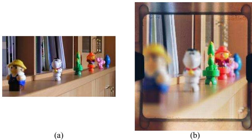
**Figure 8.** Captured IP image of real 3D scene, (a) 3D scene captured by a conventional 2D camera, (b) captured IP image exhibiting both real and virtual parts
