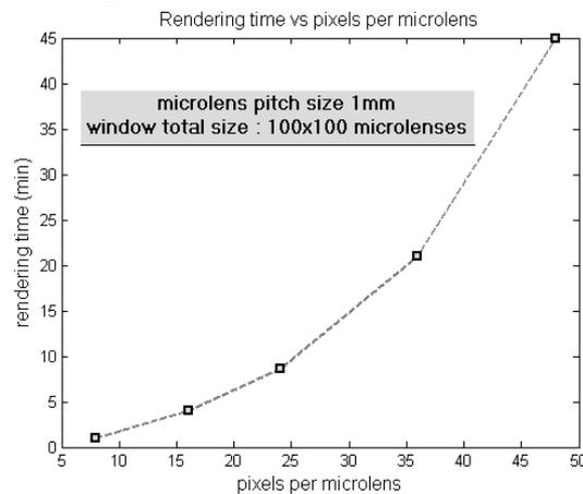
**Fig. 5.** Rendering time results versus number of pixels per microlens. A total of 100x100 microlenses are used for each render, with a square MLA of 1mm pitch without antialiasing.
