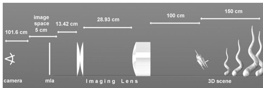
**Fig. 3.** Single stage IP capturing setup for generation of real and virtual orthoscopic images (distances and object lengths are not in scale)
