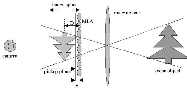
**Fig.1.** Single stage IP capturing setup for production of real and virtual images (distances not in scale).
