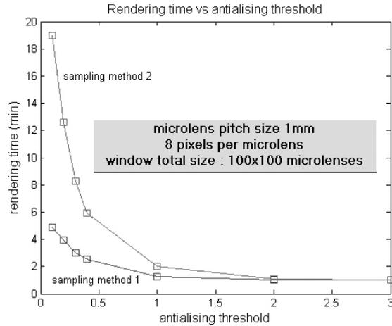
**Fig. 6.** Rendering time versus antialiasing threshold. A total of 100x100 microlenses were used for each render. A rectangular MLA was used with 1mm pitch. The sampling method 1 was an adaptive, non-recursive, super-sampling method. The sampling method 2 was an adaptive, recursive, super-sampling method with control over the maximum number of samples taken for a super-sampled pixel (we have set the corresponding depth-control parameter to 3).
