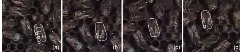
Fig. 7. Tracking Results - Sequence without blobs:aHMT, 50 particles, frames 1,15,30,50. The blob models, although initialized in (a), are quickly discarded because the background contains similar colors that distract it. In (c), the spot models are also discarded and only the contour is used. In (d), several new spots are detected.
