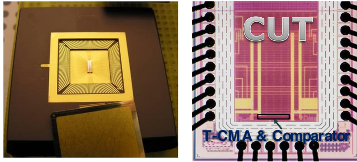
Fig. 12. Fabricated I_{DDQ} test chip and a microphotograph
