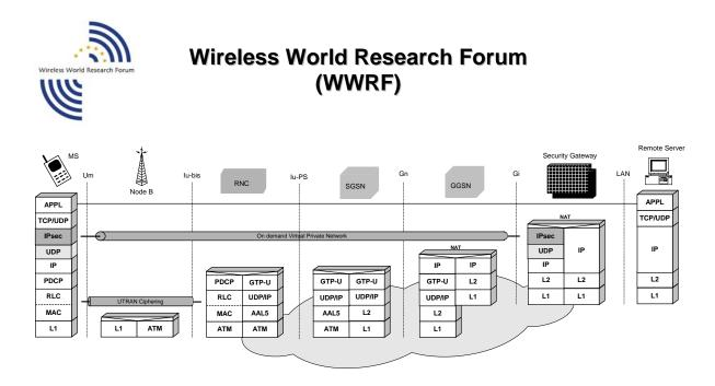
Figure 4: End-to-end VPN deployment scheme over UMTS
