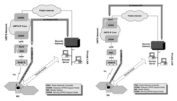
Figure 6.a: Network-wide VPN deployment scheme
