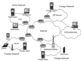
Figure 1 An All-IP network that federates several wired and wireless access technologies.
