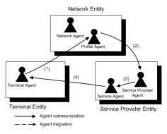
Figure 5 Service activation procedure.
