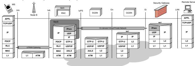
Figure 3: Protocol stack for the proposed mobile VPN scheme
