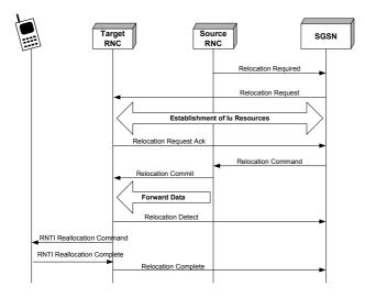
Figure 5: Intra-SGSN relocation procedure
