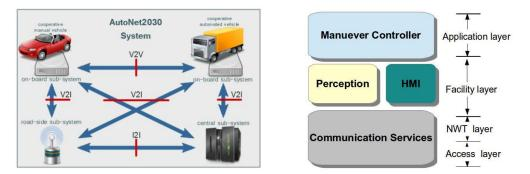
Figure 1 - Left: The AutoNet2030 system and its communication links. Right: Main components of the on-board AutoNet2030 system.
