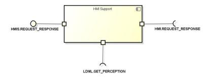
Figure 2 – Design and associated interfaces for the HMI Support module
