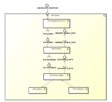
Figure 3 - Design and associated interfaces for the HMI Management module
