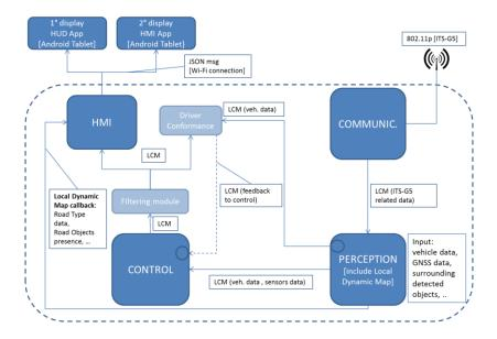
Figure 4 - Modules interaction in the AutoNet2030 architecture
