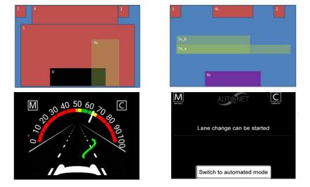
Figure 7 - Sub-areas affected and visual objects displayed in response of a specific directive (HUD: left and Secondary Display: right).
