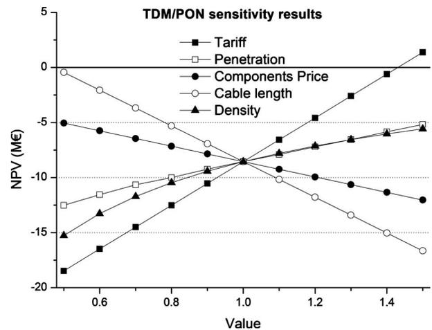
Fig. 6. Sensitivity for TDM/PON.
