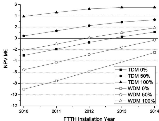
Fig. 9. NPV of the TDM/PON and WDM/PON solution depending on duct availability in the access network (80% present at main network).
