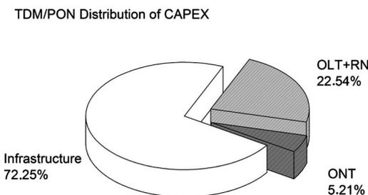
Fig. 11. Distribution of investments for the TDM/PON solution.
