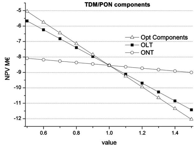
Fig. 12. Sensitivity analysis of the NPV of the TDM/PON with respect to the initial price of the optoelectronic components.
