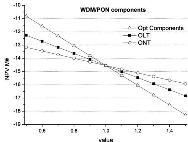
Fig. 13. Sensitivity analysis of the NPV of the WDM/PON with respect to the initial price of the optoelectronic components.
