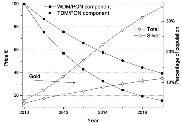
Fig. 5. Price curves for optoelectronics components and demand forecast.
