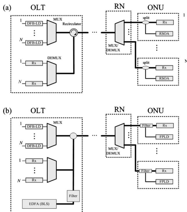
Fig. 2. Colorless ONT-based WDM/PON architectures considered in this paper: (a) reflective SOA and (b) injection-locked FPLD. EDFA, erbium-doped fiber amplifier; BLS, broadband light source.
