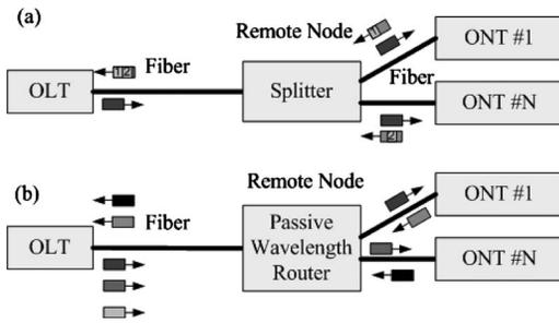
Fig. 1. PON architecture: (a) TDM/PON and (b) WDM/PON.
