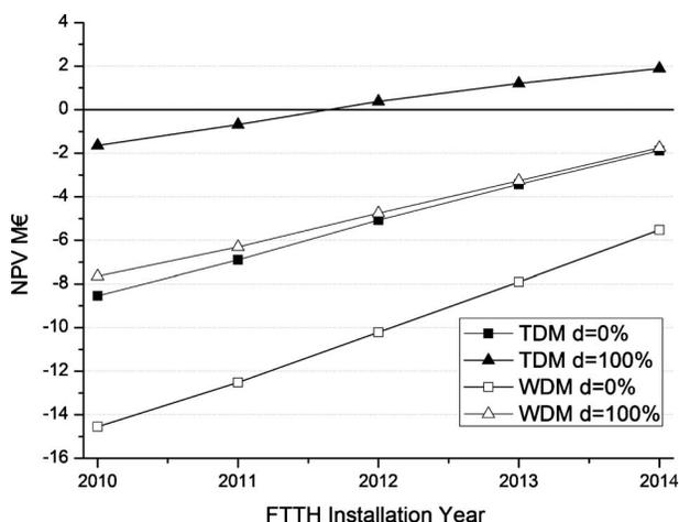
Fig. 8. NPV of the TDM/PON and WDM/PON solution depending on duct availability in the main network.
