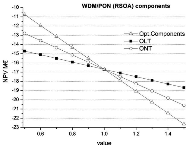
Fig. 14. Sensitivity analysis of the NPV of the WDM/PON RSOA with respect to the initial price of the optoelectronic components.
