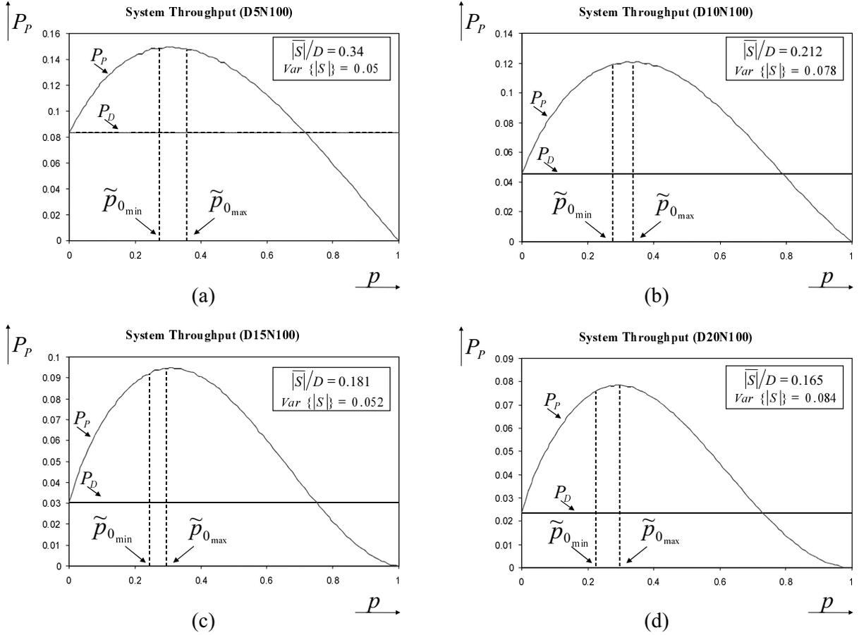
Fig. 9. System throughput simulation results for different values of  $p$  (small topology density values  $\overline{|S|}/D$ ), for both the Deterministic Policy and the Probabilistic Policy.
