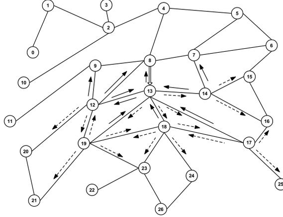
Fig. 2. Transmission sets  $\Phi_{8 \rightarrow 13}$  and  $\Theta_{8 \rightarrow 13}$  for an example network of 27 nodes.
