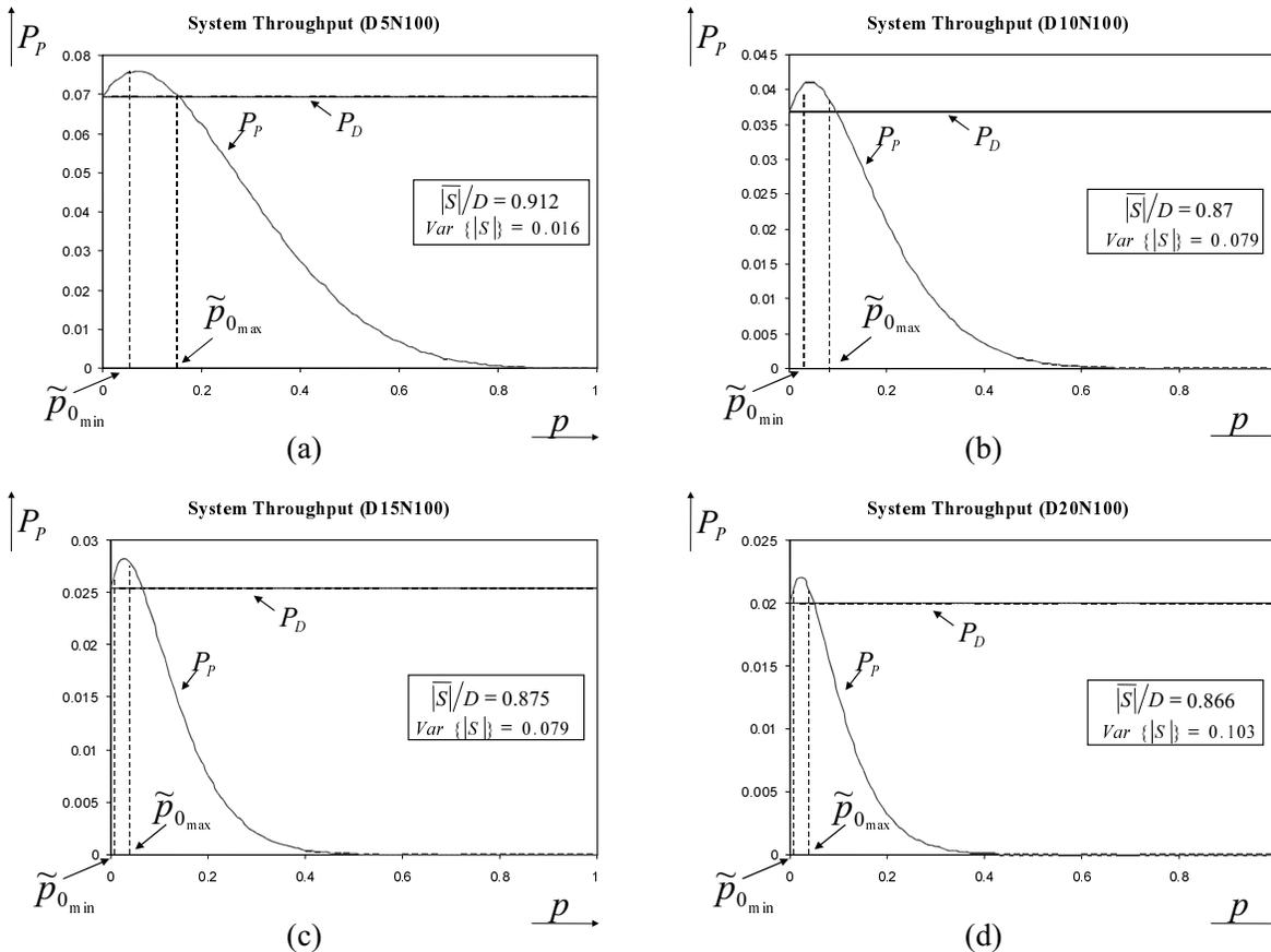
Fig. 11. System throughput simulation results for different values of  $p$  (high topology density values  $\overline{|S|}/D$ ), for both the Deterministic Policy and the Probabilistic Policy.
