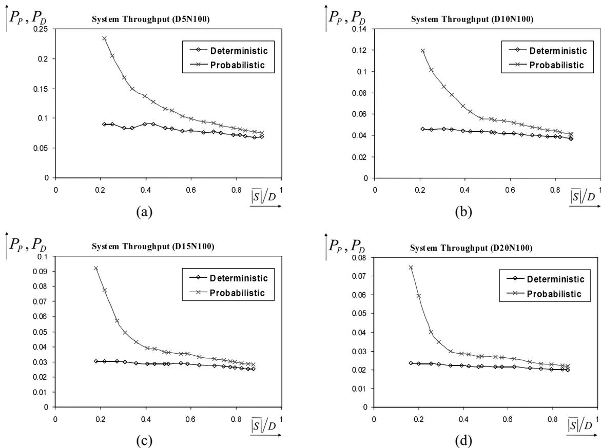
Fig. 12. System throughput simulation results, for both policies, for different values of the topology density  $\overline{|S|}/D$ .
