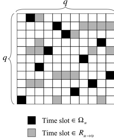
Fig. 3. Example sets  $\Omega_u$  and  $R_{u \rightarrow v}$  for node  $u$  and transmission  $u \rightarrow v$  respectively (frame size:  $q^2 = 121$ ).
