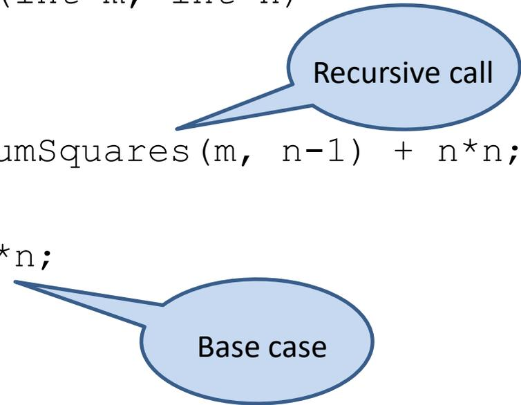
The diagram features two blue speech bubbles with black outlines. The first bubble, labeled "Recursive call", has a tail pointing to the line `return SumSquares(m, n-1) + n*n;` in the code. The second bubble, labeled "Base case", has a tail pointing to the line `return n*n;` in the code.
