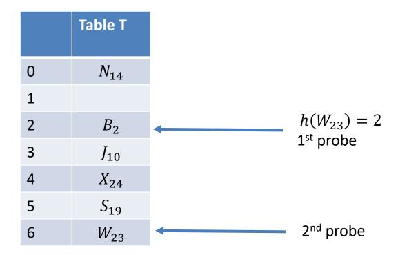
We use a probe decrement of  $p(W_{23}) = 3$ . In general probe decrements will be **different** for different keys. Try inserting key  $P_{16}$  on your own.
