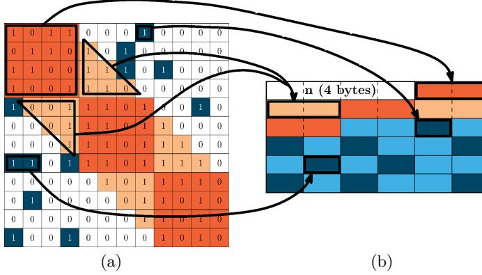
Fig. 1: Example of an adjacency matrix (a) and the corresponding compressed file format (b).
