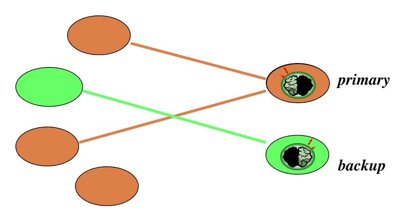
Some clients still connected to primary, but one has switched to backup and one is completely disconnected from both
