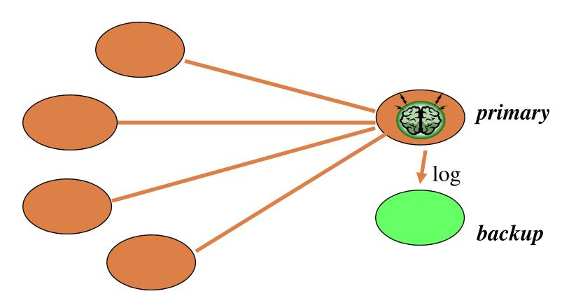
Clients initially connected to primary, which keeps backup up-to-date. Backup collects the log
