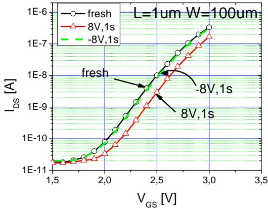
**Fig. 7.** Drain-Source current vs Gate-Source bias characteristic of a Ge nanocrystal memory cell after charging with  $\pm 8V$ , 1s write-erase pulses .
