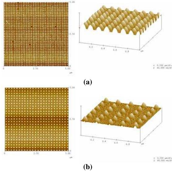
**Fig. 4.** AFM plan views and corresponding 3-D expanded images of arrays of Ge/Si heteronanocrystals grown on arrays of holes in SiO<sub>2</sub>. The lithography pitch in (a) was 150 nm while in (b) it was 200 nm. The mean dot size in (a) was 95 nm, while in (b) it was 90 nm.
