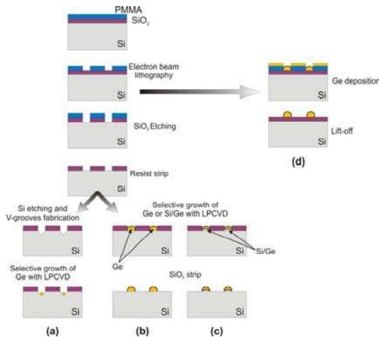
**Fig. 2.** Process flow chart for the fabrication of ordered Ge nanocrystals. (a) In V-grooves, (b) and (c) in plain windows in  $\text{SiO}_2$  and (d) with lift-off.
