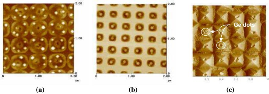
**Fig. 3.** AFM images of Ge islands grown in Si V-grooves. In (a) 3 to 4 dots were grown per V-groove (500nm V-groove opening). In (b) the V-grooves were smaller (270nm) and one large dot was formed per groove, with one smaller dot attached to it in some cases. In (c) we see an inverted image of a V-groove, 200nm large , where one dot per groove is identified.
