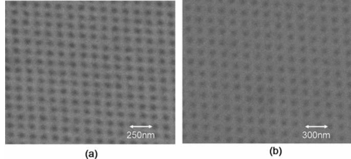
**Fig. 1.** SEM micrograph of ordered arrays of holes in PMMA. In (a) the pitch was 125nm and in (b) 150nm.
