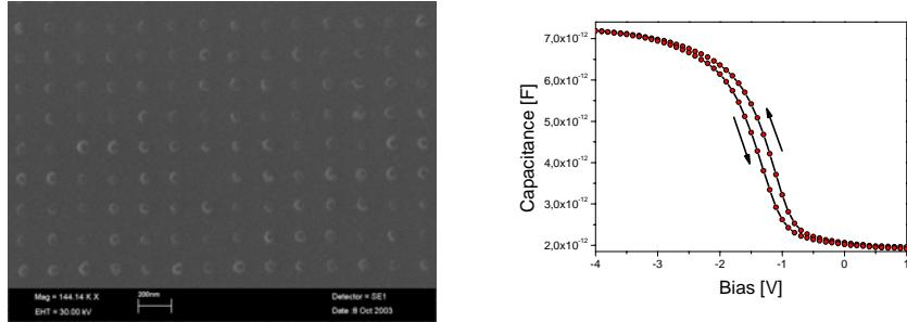
**Fig. 5.** (a) SEM image of Ge dots grown on tunneling SiO<sub>2</sub> layer. (b) Capacitance-Voltage measurements of capacitors containing arrays of Ge dots. A clear hysteresis effect is present.
