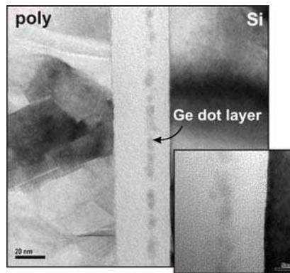
**Fig. 6.** Cross sectional TEM image of the Ge layer within SiO<sub>2</sub>
