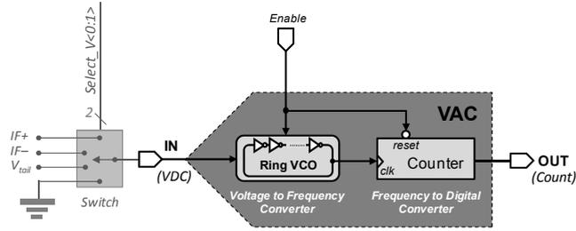
**Fig. 5.** Voltage acquisition circuit (VAC)
