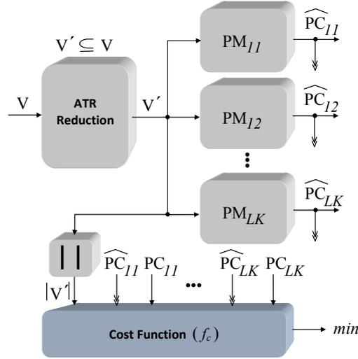
**Fig. 8.** Principle of ATR reduction (global approach)
