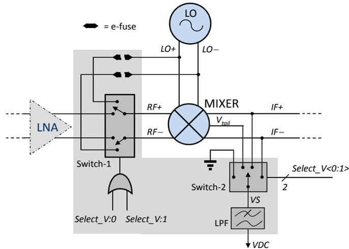
**Fig. 6.** RF mixer design modifications (shaded area)
