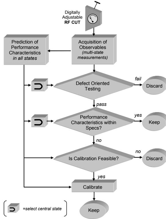
Fig. 1. Testing and calibration flow
