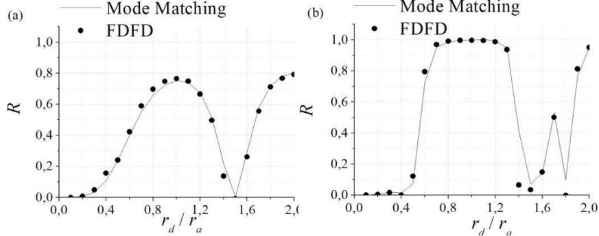
**Fig 1.** Comparison of power reflection coefficient of the MM and the finite difference frequency domain (FDFD) methods for a) single, and b) triple defect rods inside a PCW.
