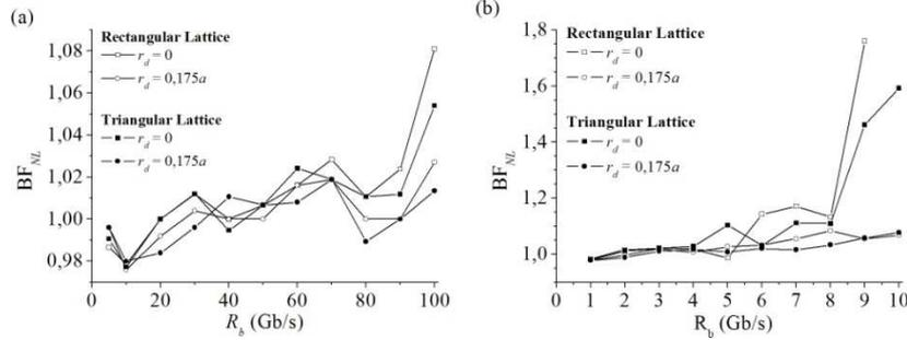
**Fig 8.** Broadening factors for bright solitons propagation in various geometries of PCWs obtained at a specified delay of either a)  $T_d=1$ ns for signals up to 100Gb/s and b)  $T_d=5$ ns for signals up to 10Gb/s.
