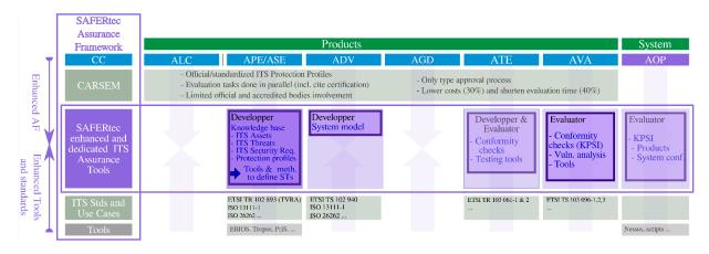
Fig. 3. The SAFERtec Security Assurance Framework (SAF): introduced evaluation tools beyond Common Criteria
