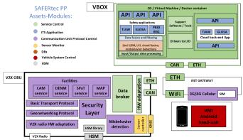
Fig. 3. Distribution of system components of the SAFERtec bench to high level assets of the SAFERtec architecture
