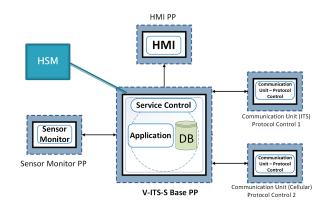
Fig. 1. The Modular Protection Profile architecture - a PP configuration
