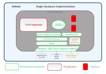
Fig. 2. (a) V-ITS-S as an integration of multiple interconnected components (b) V-ITS-S as a Single Hardware/Software unit
