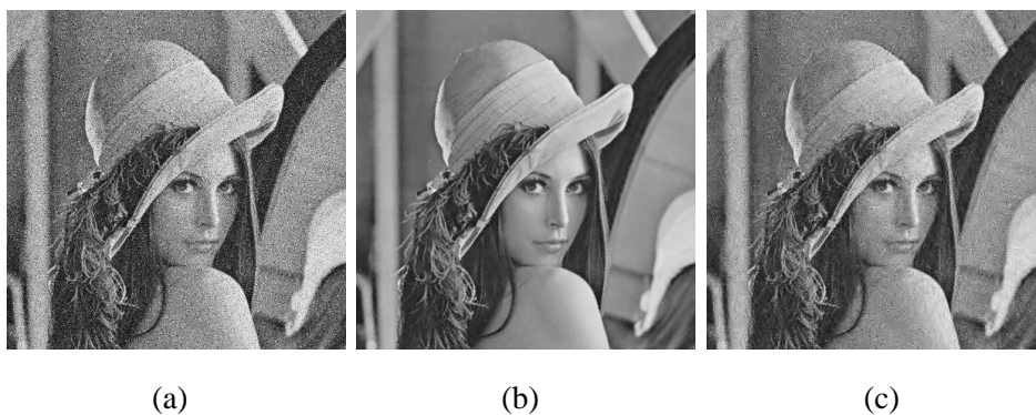
Fig. 5. (a) Lena corrupted by 20% of impulse noise of type II, (b) denoising using the kernel approach (PSNR=35.27 dB), (c) denoising with BiShrink (PSNR=22.83 dB).
