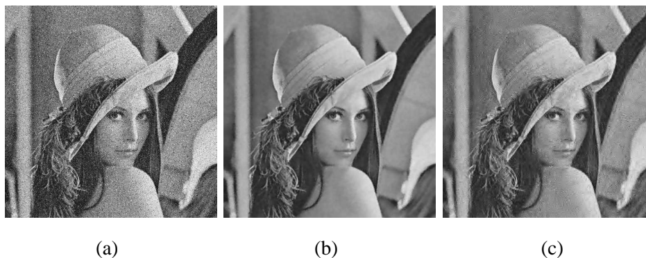
Fig. 15. (a) Lena corrupted by gaussian noise with s = 10 and 20% of impulse noise of type II ( a = 128 ), (b) denoising using the kernel approach (PSNR=32.27 dB), (c) denoising with BiShrink (PSNR=25.30 dB).
