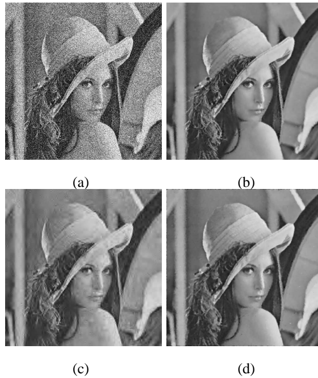
Fig. 6. (a) Lena corrupted by 50% of impulse noise of type II, (b) denoising using the kernel approach (PSNR=30,71 dB), (c) denoising with BiShrink (PSNR=26.41 dB), (d) denoising with the median filter of MatLab (PSNR=28.08 dB).
