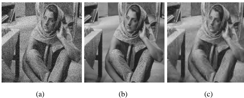
Fig. 8. (a) Barbara corrupted by 40% of impulse noise of type II, (b) denoising using the kernel approach (PSNR=24,81 dB), (c) denoising with BiShrink (PSNR=24.28 dB).
