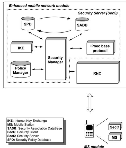
Figure 2: Security Client (SecC) and Security Server (SecS) modules
