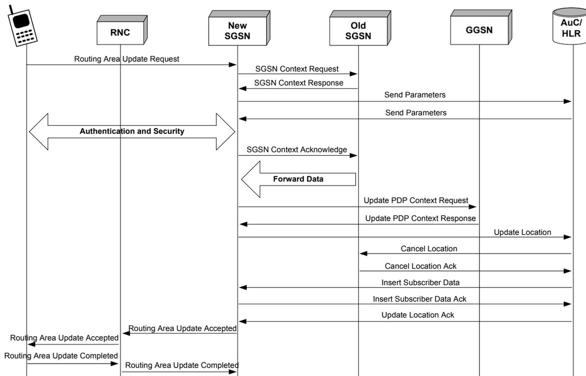
Figure 6. Inter-SGSN routing area update procedure
