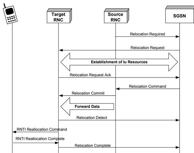
Figure 5: Intra-SGSN relocation procedure
