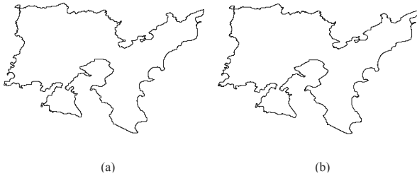
Figure 4. (a) Coastline D (Lemnos) consisting of 7186 points. (b) The reconstructed curve using the Method 1 with comp. ratio = 1:5.00
