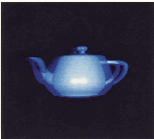
Plate 7. 3D image simulation: perspective proj., size = 4x , distance = 4y
