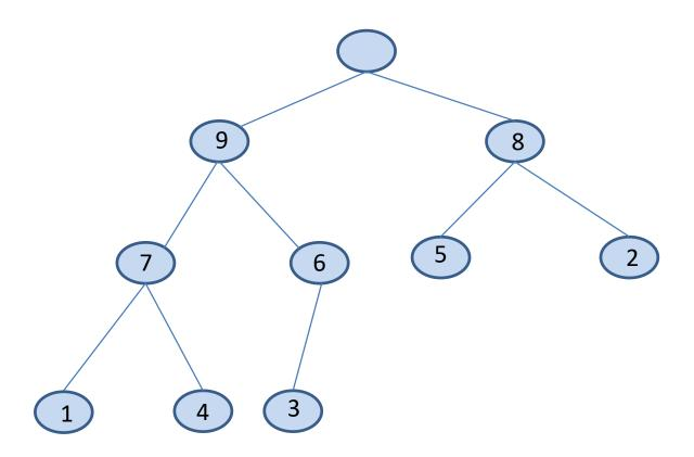
Delete the node with value 3 and insert this value into the root.
