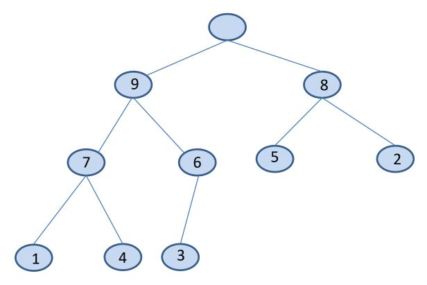
The Remove function optimizes our earlier method by moving 9, 7 and 4 upward to make a hole where 3 will come to be inserted.
