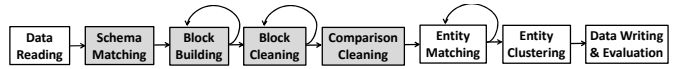
Fig. 2. One of pyJedAI ’s pipelines for batch ER. Gray rectangles indicate optional steps. Self-loops show that multiple methods can be selected per step.
