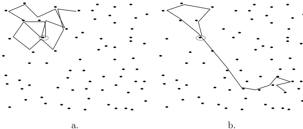
Fig. 1. An agent (starting from the initiator node depicted in dotted ellipsis) under: (a) the RW mechanism and (b) the J-RW mechanism.
