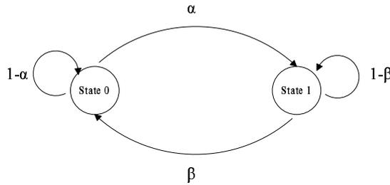
Fig. 2. Markov chain mechanism for controlling J-RW agent movements.
