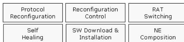
Figure 3-1: Functional Entities of RCM. RAT and NE are abbreviations of Radio Access Technology and Network Element respectively.
