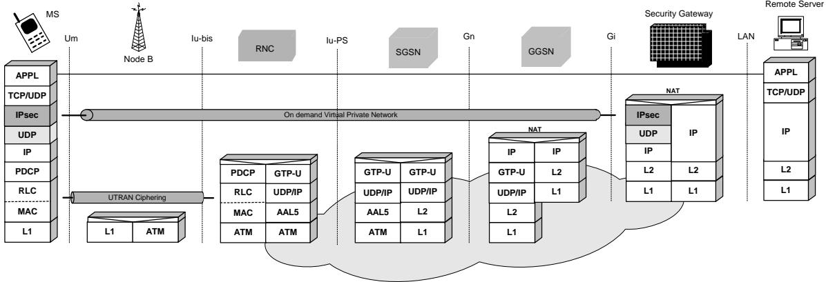
**Figure 4:** End-to-end VPN deployment scheme over UMTS
