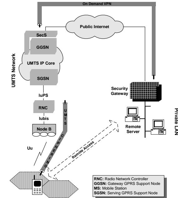
**Figure 6.b:** Border-based VPN deployment
