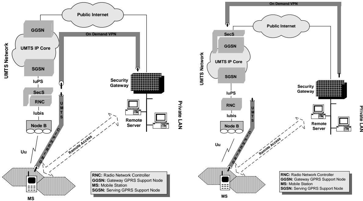
**Figure 6.a:** Network-wide VPN deployment scheme
