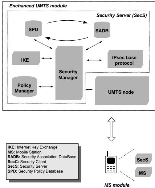
**Figure 5:** Security Client (SecC) and Security Server (SecS) modules
